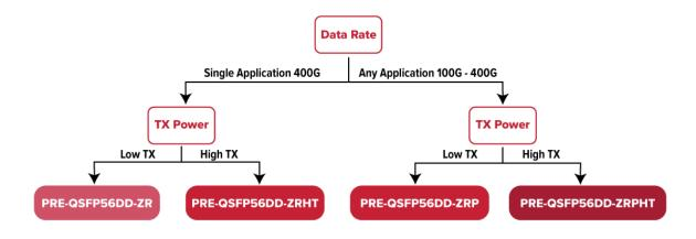
Figure 6. 400G ZRx Transceiver Decision Map – DWDM/Amplified Link
