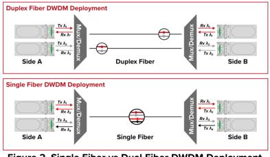
Figure 2. Single Fiber vs Dual Fiber DWDM Deployment
