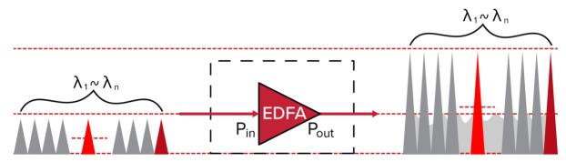
Figure 4. Visual Representation of Amplification using an EDFA
